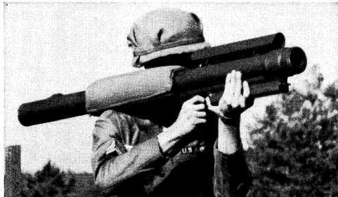
Redeye, U.S. army surface-to-air missile. The 20-lb. anti-aircraft missile is fired from a bazooka-type launcher
