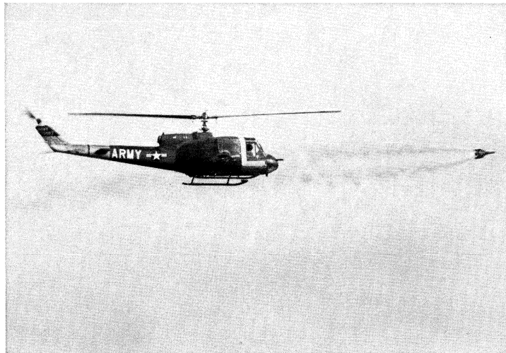
SS-11, French surface-to-surface, wire-guided missile, after being launched from a U.S. army helicopter. The short-range, antitank missile is visually tracked and can be launched from the ground as well as from a helicopter
