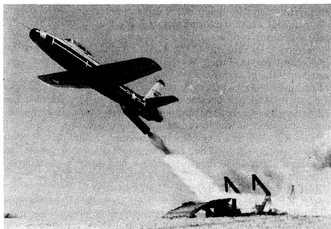
FIG. 5.—A SOLID-PROPELLANT ROCKET, ATTACHED BENEATH THE TAIL OF A U.S. AIR FORCE F-84 FIGHTER PLANE. BOOSTS THE AIRCRAFT INTO THE AIR FROM A ZERO-LENGTH LAUNCHER. ELIMINATING THE NEED OF A GROUND TAKE-OFF RUN
