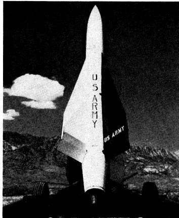
Hawk, surface-to-air missile of the U.S. army and marine corps designed to intercept low-flying aircraft
