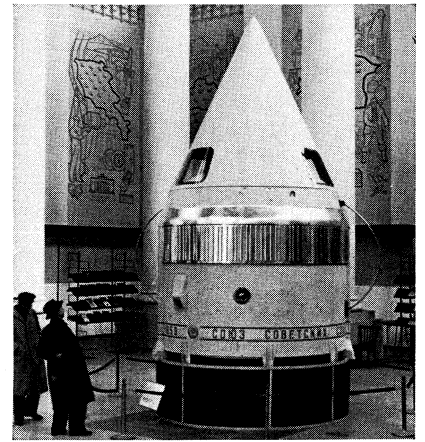
Model of last stage of Lunik I, Soviet lunar probe which was launched Jan. 2, 1959. The 3,245-lb. satellite entered into orbit around the sun after passing near the moon
