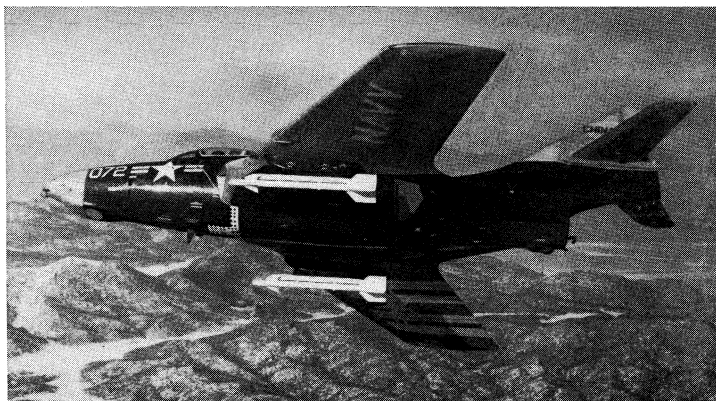
Navy F9F-8 jet fighter equipped with Sidewinders, 9-ft., 155-lb. air-to-air missiles with heat-homing guidance system; range is about 3 mi. Also used by the air force
