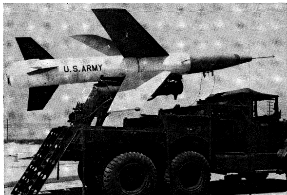
Lacrosse, a short-range surface-to-surface missile of the army designed for tactical use in field support
