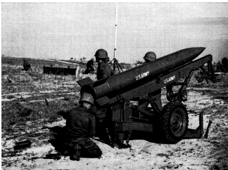
Little John XM-51 being readied for firing. An unguided surface-to-surface rocket, it is used by the U.S. army for field support. Range, 10 mi.
